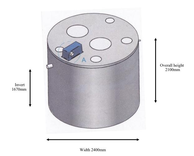
**HOLE WIDTH SOULD BE NO LESS THAN 3000mm TO REMOVE LIFTING LUGS**
